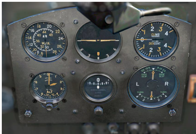
Figure 50,: Blind-flying panel (late model)
