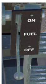
Figure 82: Main fuel valve
