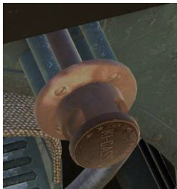
Figure 83: Engine primer pump
