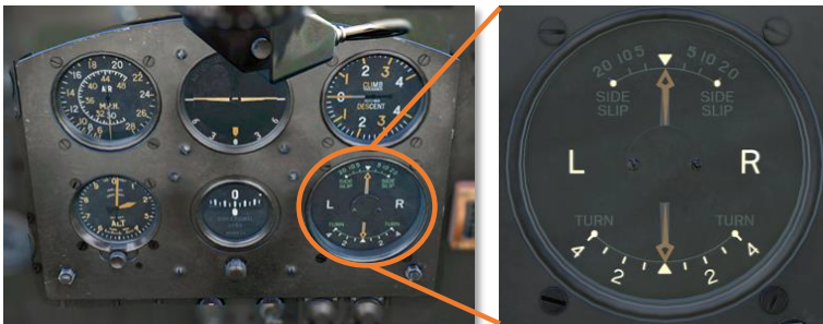
Figure 58: Sideslip indicator
