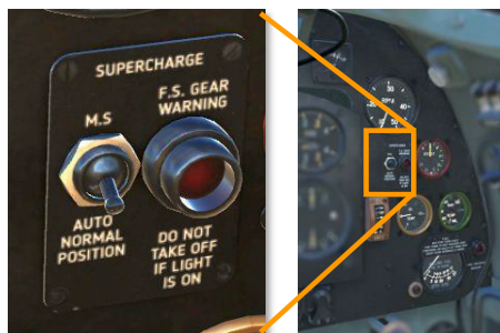
Figure 71: Supercharger control panel
