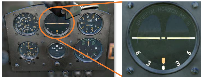
Figure 53: Artificial horizon
