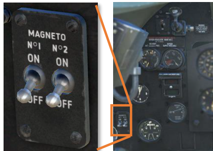
Figure 67: Magneto switches
