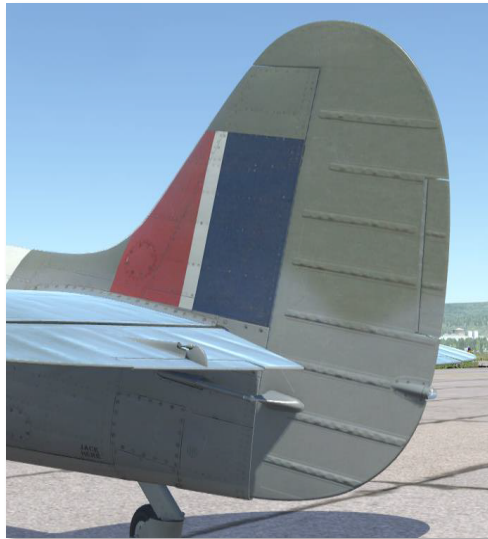
Figure 30: Rudder and tail unit
